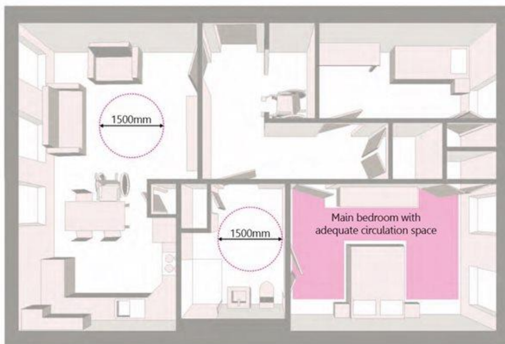
Figure 5.11: Circulation space within wheelchair accessible apartment
